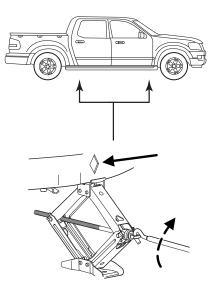
**WARNING:** To lessen the risk of personal injury, do not put any part of your body under the vehicle while changing a tire. Do not start the engine when your vehicle is on the jack. The jack is only meant for changing the tire.
